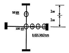
3. A truss system consisting of six bar elements is shown below. The modulus of elasticity of all the elements in this truss system is E= 200GPa. The cross-sectional areas all Members are given as A1 = 0.010m<sup>2</sup>. Calculate the member forces and stiffness matrix.
