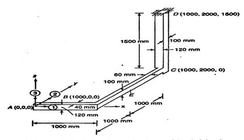
5. Using Tension coefficient method calculate the member forces of the pin jointed space truss as shown figure below. [8]
