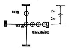
3. A truss system consisting of four bar elements is shown below. The modulus of elasticity of all the elements in this truss system is E= 29.5 × 106 N/mm2. The cross-sectional areas are given as A1 = 0.8mm2, A2 = 1 mm2, A3 = 1.2 mm2 and A4 = 1.1 mm2.. Developed sriffness matrix and calculate the member forces.
